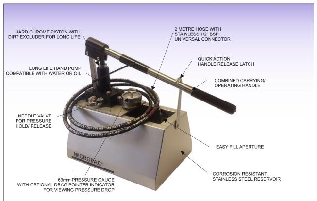
TYPICAL APPLICATIONS: PRESSURE AND HYDROSTATIC TESTING OF SYSTEMS AND PIPEWORK ON SITE OR IN-HOUSE. WATER OR OIL DUTY. PRESSURES UP TO 60 BAR
